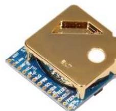
図－7 S-300L-3V(CO<sub>2</sub>計)
